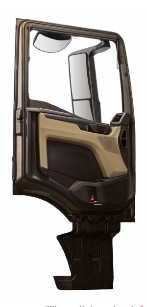
With a very wide door opening angle of 89 degrees and the very low step position, the new MAN TGS clears the way for getting in and out ergonomically, whether you are at a parking lot or on a building site.
